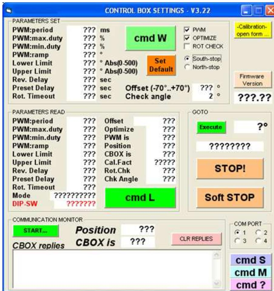
Figure 1-3 An example of a bad user interface, maybe designed thinking in a hardware expert, but to provide software like this to the end users is not good [BuiG08]
