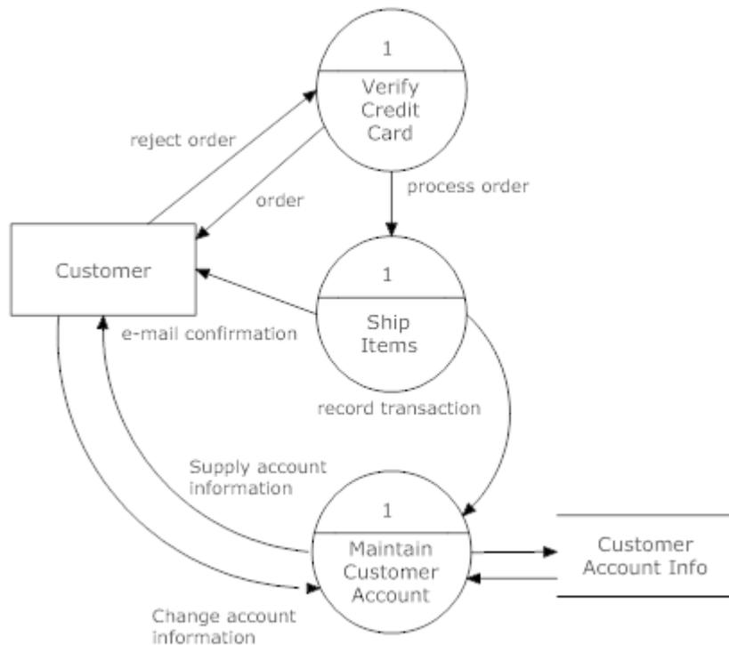
**Figure 2-2 Example of how to use the Yourdon & Coad notation for data flow diagrams**
