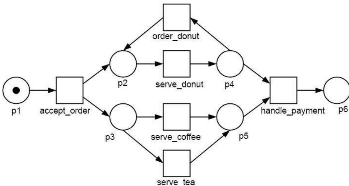
Figure 2-5 Petri net modelling the simplified workflow of a waiter in a cafe [vand01]
