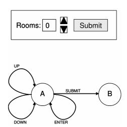
Figure 7.10 Room reservation form and corresponding state machine.
