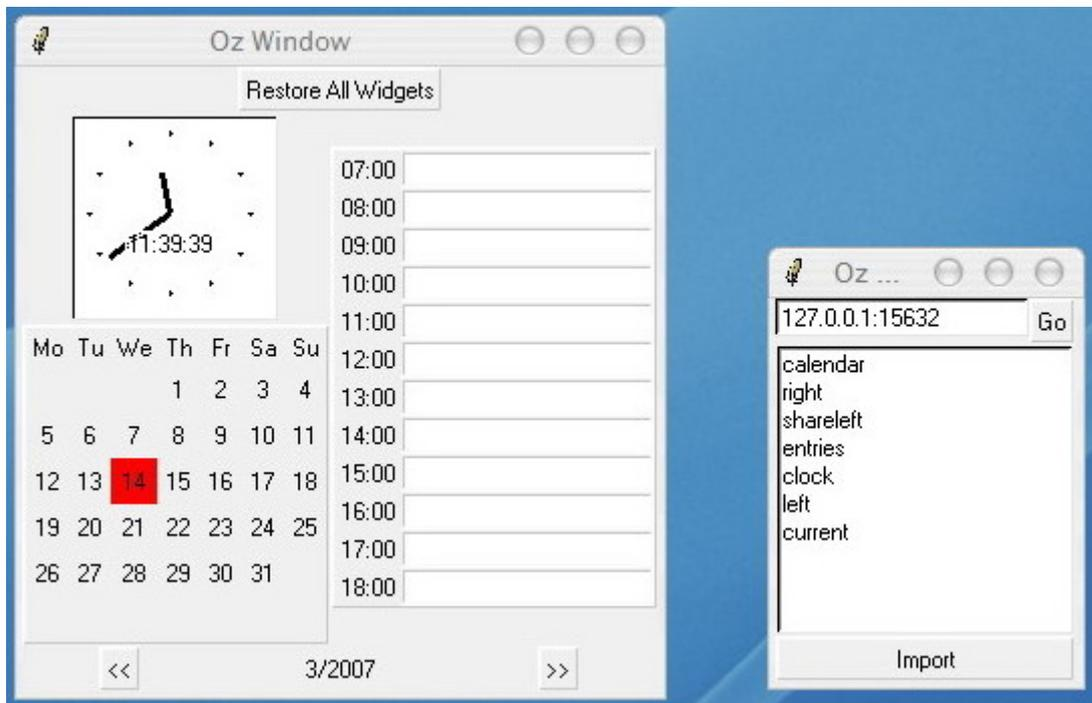
The Calendar application at the left offers different parts of its UI using the EBL discovery module. The UniversalReceiver application at the right gets the information over these parts. One can select one of them, and import it.
