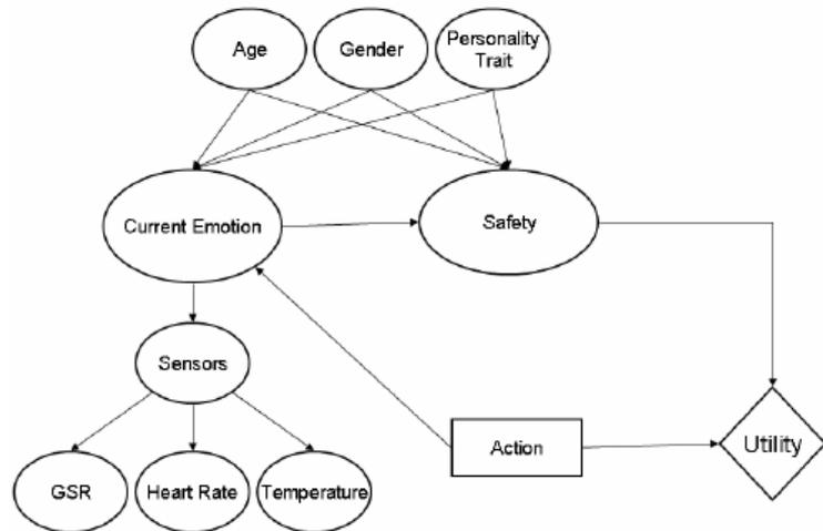
**Figure 28 – Bayesian Belief Network representation of Driver Model (NASOZ & LISETTI, 2007)**
